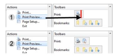
To remove an action from a Toolbar, click the action in the Toolbar and with the mouse button pressed down, drag the mouse out of the window (see 1 below) until the mouse cursor changes to a circle with a slash or an X.
