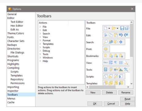
The Toolbar Options dialog is used to to control which operations appear in the application Toolbars (see <u>Using Tool Bars</u> for more information). Open the Toolbar Options dialog by clicking 'Tools > Options...' and selecting *Toolbars* from the list or by right-clicking on a Toolbar and selecting *Customize...*.
